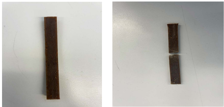
Figure 26. Rectangle composite before and after Flexural testing.
